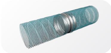
For preventing back draft when the ventilation system is not active. Wings of the back-draught shutter inside the connector open under the pressure created by the airflow. Then they automatically close with the spring work. Connector is made of galvanized steel. Back-draught shutter wings are made of sheet aluminium.
