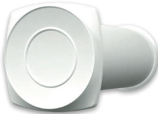
Supply valve is designed for fresh air supply in premises with forced ventilation systems. The device consists of a duct with thermal and sound insulation, and filtering elements. Ends up with a grille on the outside, and with an adjusting shutter on the inside.
