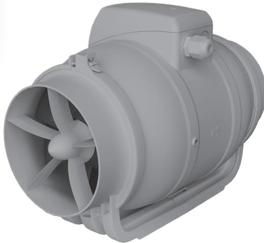
Axial inline mixed-flow fans are designed for supply-exhaust ventilation systems of residential, public and industrial buildings. Fan's body, a central part with the motor, impeller and implemented terminal box, is detachable and allows easy maintenance. It is fastened to the nozzle parts with hose clamps.
