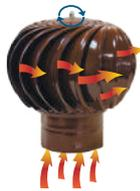
Rotary turbine vent increases air draught in the ventilation duct, encouraging better air exhaust. Protects the air duct from the unintentional outside elements (leaves, dirt and precipitations) and prevents back draft. Operation is based on a natural weather processes: the stronger the wind, the better the ventilation quality.
